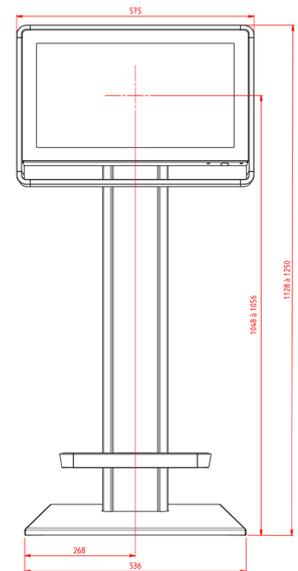
FIXATION AU SOL RECOMMANDÉE PAR CHEVILLES CHIMIQUES M10. LA TIGE FILETÉE NE DOIT PAS DÉPASSER DE PLUS DE 26 MM DU SOL.
